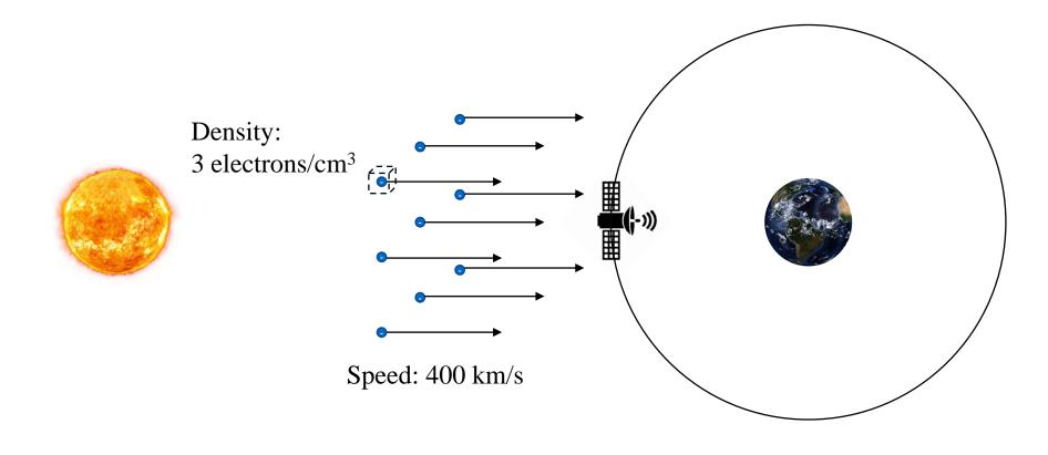
Assumption 1: The speed of the plasma around SWP CubeSat is 400 km/s, with a density of 3 electrons per cubic centimeter. These free electrons are flying in parallel from the Sun towards the Earth.
