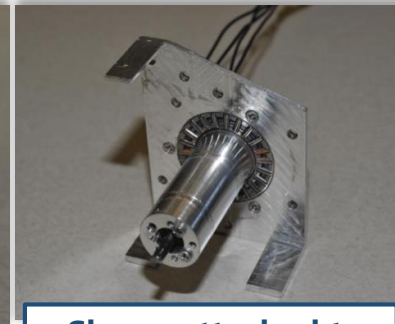
Sleeve attached to motor for later mounting
