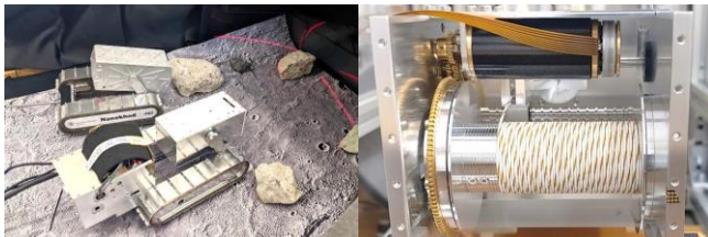
Figure 1. Left: Nanokhod Laboratory (front) and Mechanical Model (back) on a test demonstration Right: Nanokhod Tether Mechanism (right)
