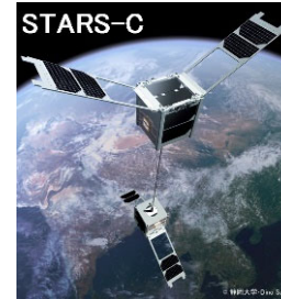
Released from the ISS in 2016 Decayed ✓ 100m long tether ✓ Kevlar tether
