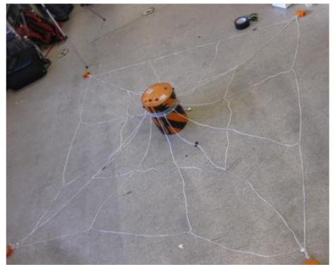
Net Rotation Unfolding (Electric Motor)
